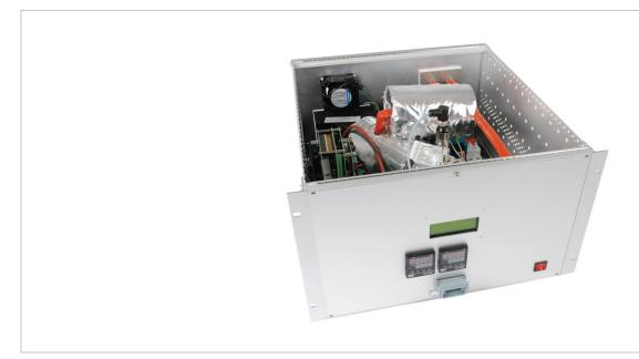
NEO Monitors Laser $Gas^{TM}$  is using Tuneable Diode Laser Absorption Spectroscopy (TDLAS) i.e. a non-contact optical measurement method employing solid-state laser sources. Therefore, the sensor remains unaffected by contaminants and corrosives and does not require regular maintenance. The laser beam is coupled into a measurement cell, where it is reflected one time from a flat mirror in order to enhance the analyzer sensitivity.
